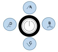
The configuration menu is activated by simultaneously pressing the buttons "up" (A), "left" (D) and "right" (B) for at least 3 seconds.
