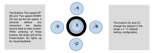
With power-button (E), the device can be set in standby mode by pressing the button (if keycard-switch function is NOT used). If the button is used as a occupancy button, the button must be pressed for at least 3s, in all other cases, a short actuation is sufficient. In standby mode, the display and all outputs are switched off (controller deactivated). The frost and heat protection monitoring remains active. **Modbus registers can still be read (e.g. room temperature).**
